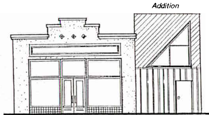
Inappropriate: The commercial addition disregards the architectural style, uses noncompatible materials and has an inappropriate fenestration pattern.
