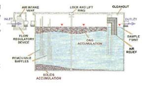
establishment that implements BMP's will realize financial benefit through a reduction in their required grease trap maintenance frequency. At a minimum, all grease traps **MUST** be cleaned at least once each week in accordance with Pinellas County Code or more often as necessary to prevent pass-through of grease and other food solids.
