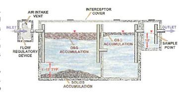
capacity of the interceptor should be such that it provides adequate residence time. Upon entering the interceptor the wastewater flow slows, which allows the lighter grease to separate from the wastewater and float to the top of the interceptor where it cools. The grease will tend to collect and rise to the surface where it accumulates until the interceptor is cleaned.
