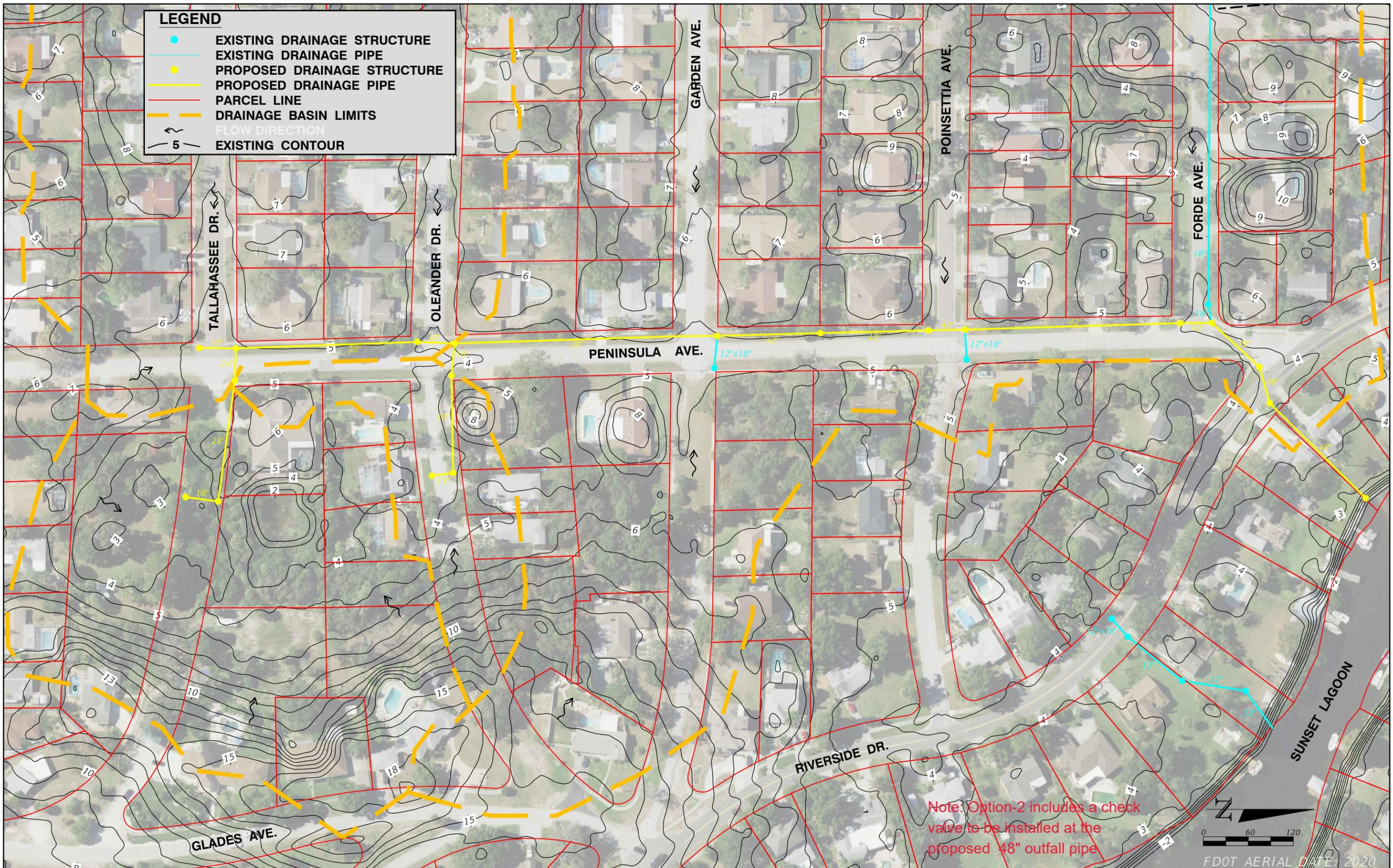
Note: Option-2 includes a check valve to be installed at the proposed 48" outfall pipe
