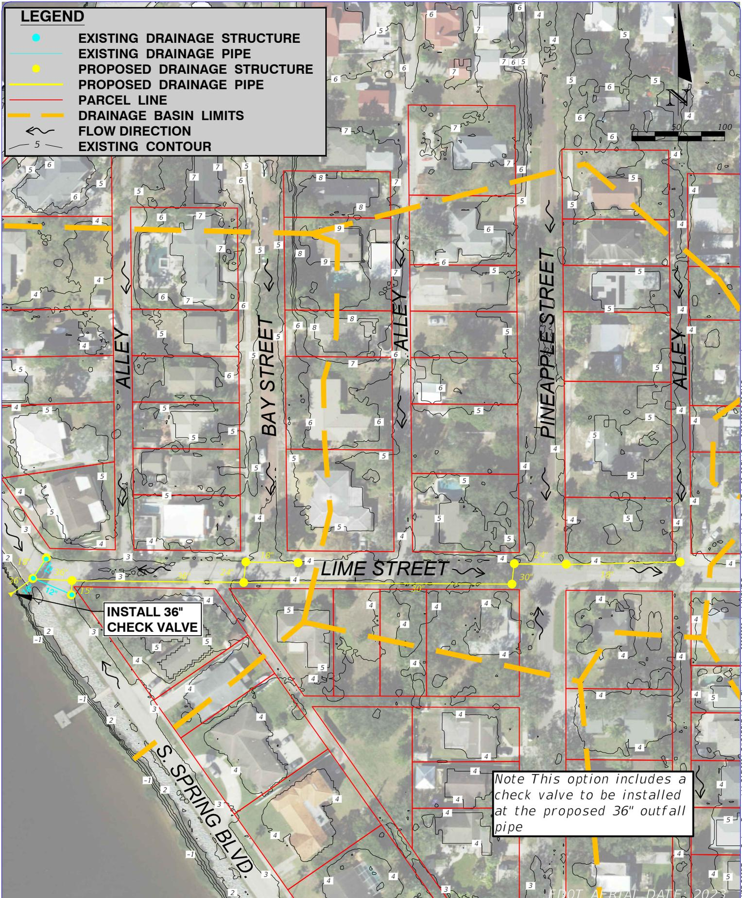
Note This option includes a check valve to be installed at the proposed 36" outfall pipe
