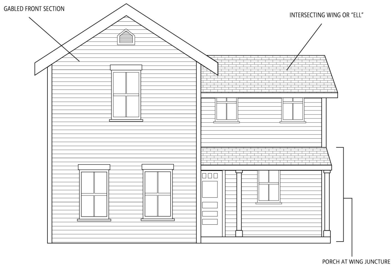
Figure 17: Diagram of a Gabled Ell building type.
