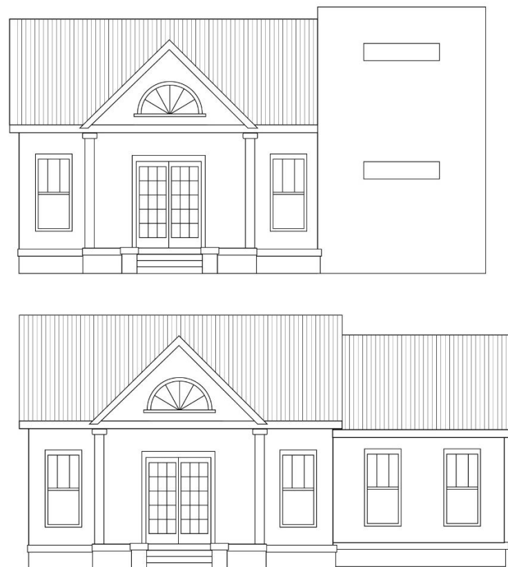
Figure 91: The top illustration shows an example of an inappropriate addition while the bottom illustration shows an example of an appropriate addition.
