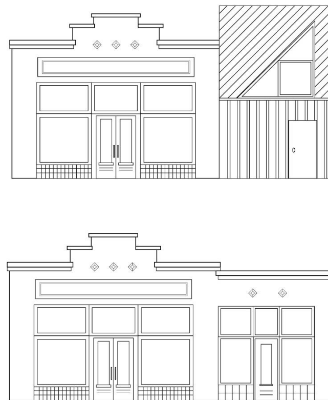
Figure 122: The top illustration shows an example of an inappropriate addition while the bottom illustration shows an example of an appropriate addition.
