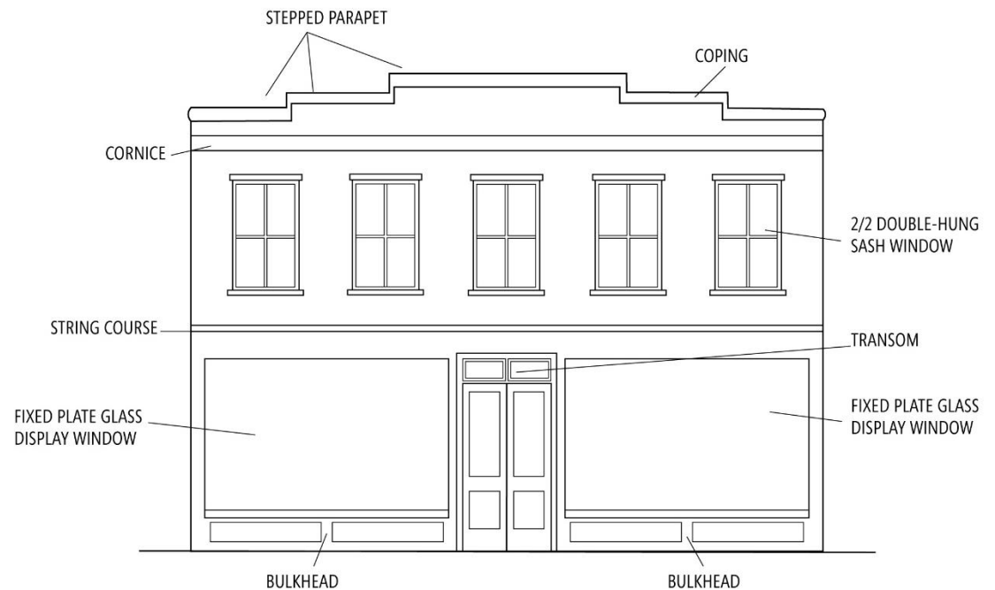
Figure 10: Diagram of a Two-Part Commercial Block Storefront
