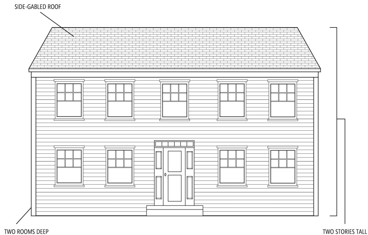
Figure 14: Diagram of a Double Pile building type.
