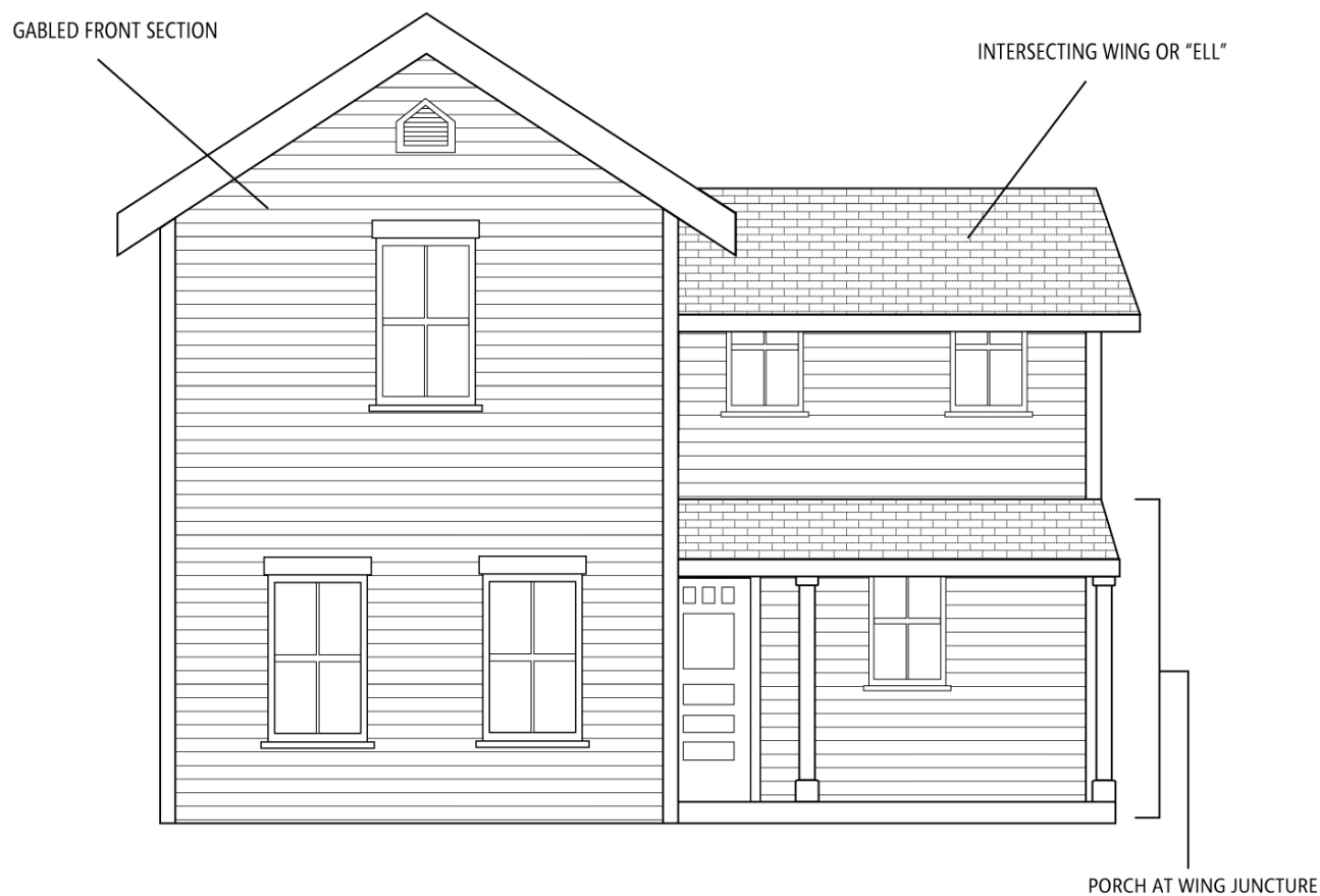
Figure 17: Diagram of a Gabled Ell building type.
