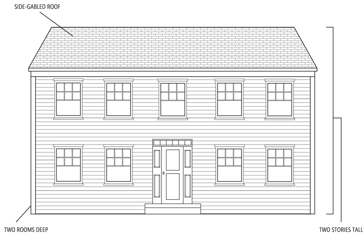
Figure 14: Diagram of a Double Pile building type.
