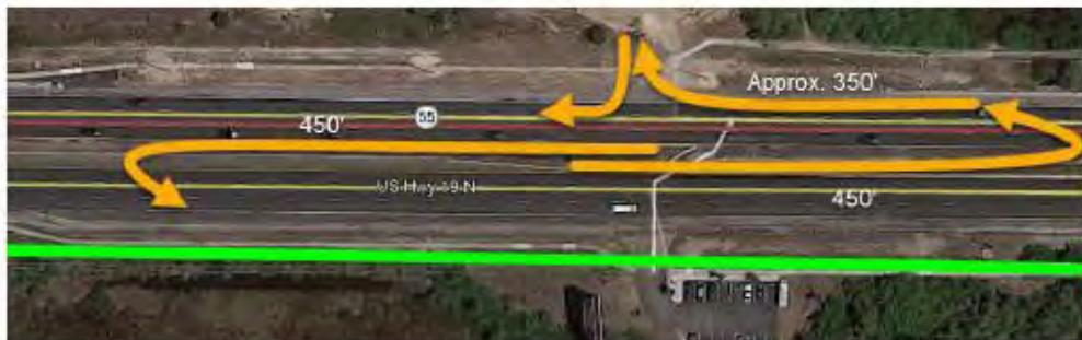
Figure 1 – Proposed Offset Left-Turn Median Opening
