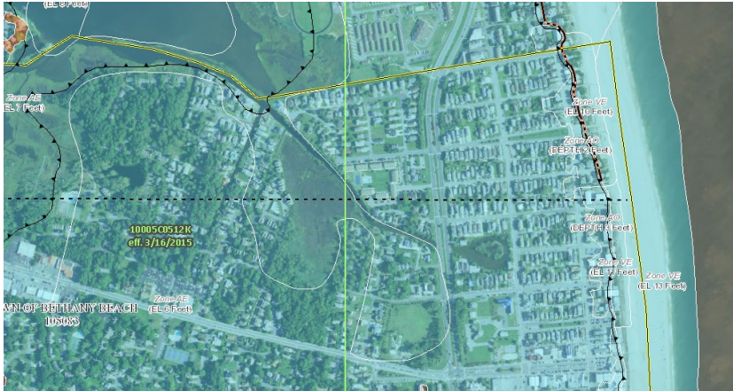
Figure 1: A flood map panel showing the Limit of Moderate Wave Action (LiMWA), indicated by the black lines with arrows. The arrows point toward the inland limit of the Coastal A Zone.
