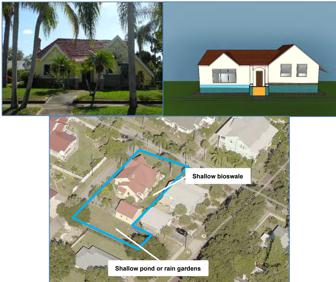
Figure 41. Residence at 409 West Lemon Street, illustrating potential coordinated protection using landscape adaptations and flood-wrapping (blue line indicates approximate property line).
