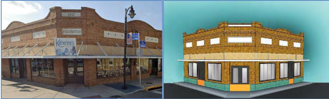
Figure 37. Temporary protective measures using floodgates and flood-wrapping for single story commercial: Gonatos Building, 628 Athens Street.
