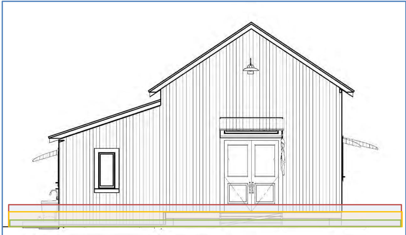
Figure 31. The National Register building, “Meres Packing House” (see Figure 12) showing the general elevation of flood waters at one (green), two (orange) and three (red) feet above grade. This building has corrugated metal walls, a pier-supported foundation, and wood floor without a sub-floor. The ground elevation at this building entrance is less than three (3) feet above sea level.
